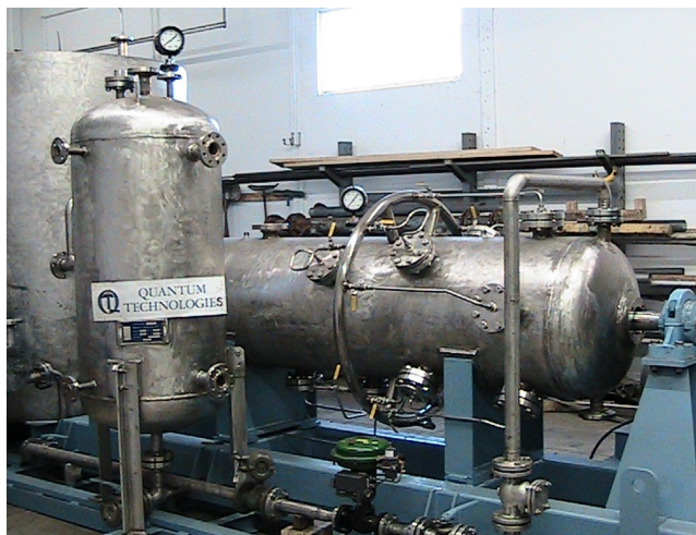
The 28" reactor and the degasser ready for shipment.
